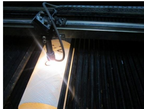
Fig. 3 Create an opening on the shell
