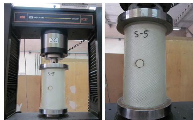
Fig. 6 A specimen prepared for buckling test
