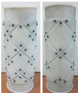
Fig. 1 The Polyethylene molds used for manufacturing the specimens
