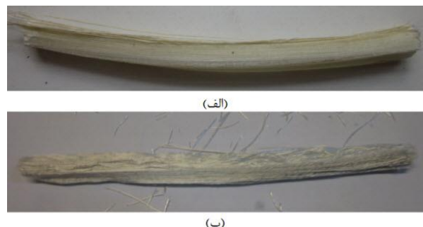
Fig. 5 A part of the rib (a) before and (b) after burning to determine volume fraction of fiber in the stiffeners
