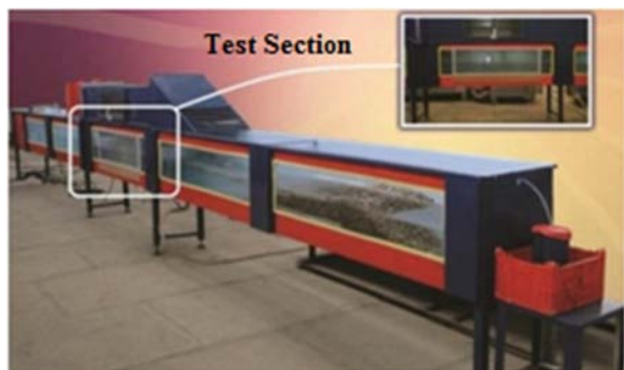
Fig. 4 A picture and scheme of bed wave maker
