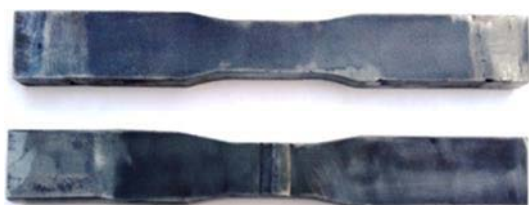
Fig. 4 Photograph of tensile test specimens
