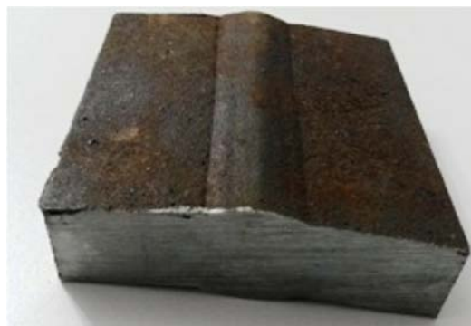
Fig. 2 Photograph of a seam weld sample cut from API X65 pipe
