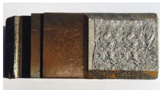
Fig. 9 Fatigue and fracture surface of CT specimen
