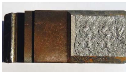
Fig. 9 Fatigue and fracture surface of CT specimen
