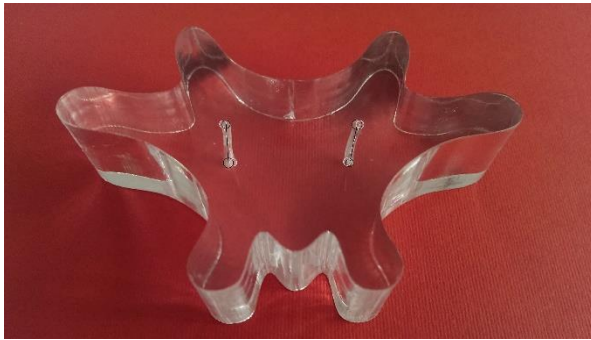
Fig. 7) The phantom made up of transparent plexiglass and shaped like the posterior view of the human lumbar vertebra with the planned holes in it. Planned holes are highlighted by black lines and created holes are highlighted by white lines.
