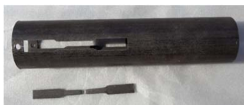
Fig. 4 figure of model for tension test
