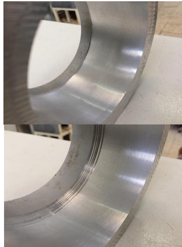
Fig. 18 Comparison of surface finish of boring operation, control off (DOC=0.2mm) and control on (DOC=2.5mm), a- Cutting test control off (DOC=0.2mm), b- Cutting test control on (DOC=2.5mm)
