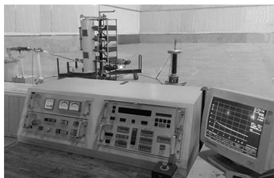
Fig. 5 Electrohydraulic forming apparatus
