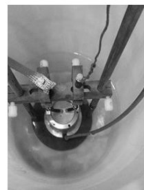
Fig. 6 Electrode system in the water chamber
