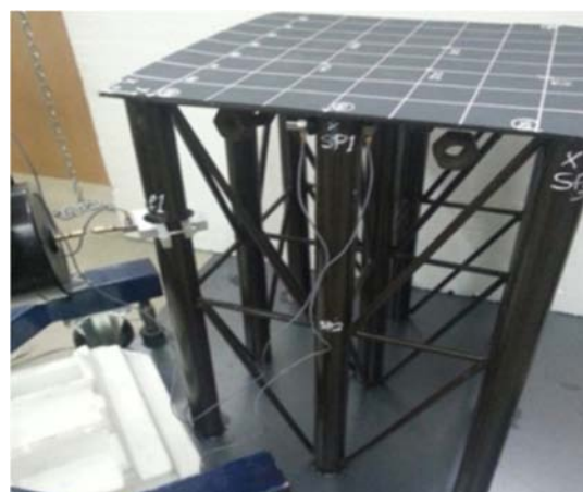
Fig. 1 The model of pier for experimental modal analysis
