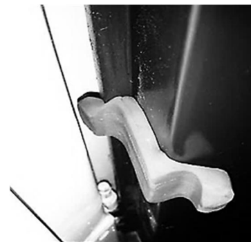
Fig. 4 The paste is sticking to the door with the same dimensions of gap
