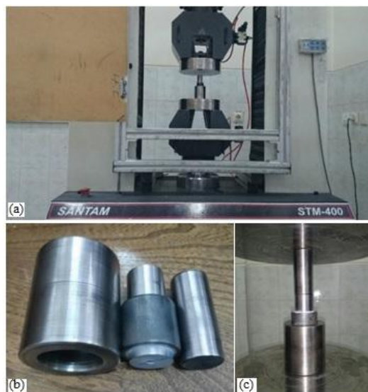
Fig. 4 Extraction process with a fixture and universal machine test. (a) Universal testing machine. (b) Designed fixture for extraction of assembled part. (c) Assembled part and designed fixture on universal testing machine during extraction
