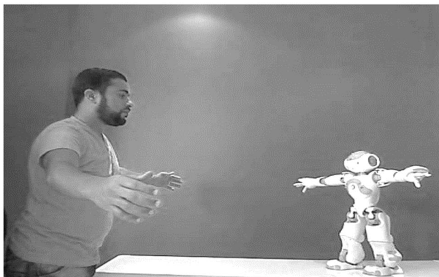
Fig. 1 Imitation learning of hand movement in humanoid robot [1]
