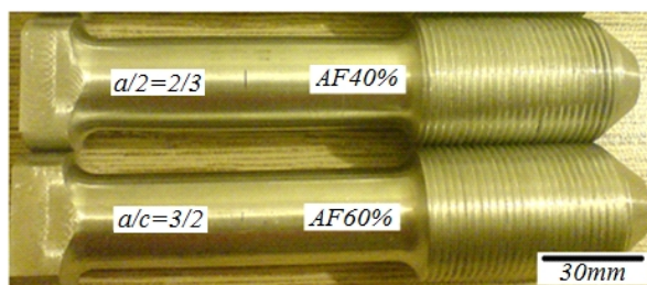
Fig. 5 Two samples of cracked specimens with \xi = 0.4
