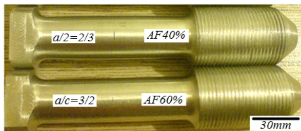
Fig. 5 Two samples of cracked specimens with \xi = 0.4
