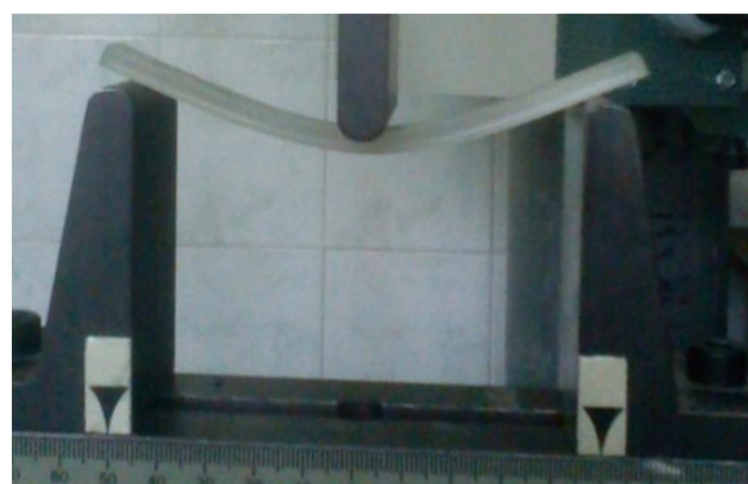
Fig. 2 Configuration of three-point bending test
