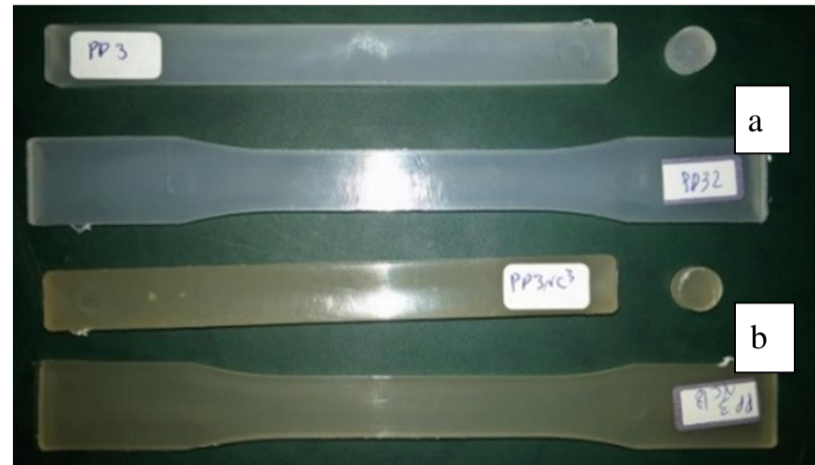
Fig. 1 Tension, compression and bending specimens a- PP b- PPNC3
