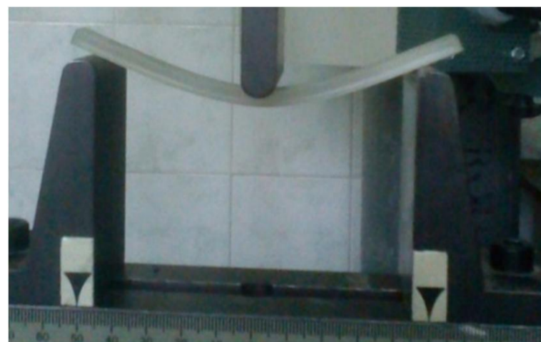
Fig. 2 Configuration of three-point bending test
