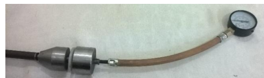
Fig. 9 Pressure gauge connection to the main axle
