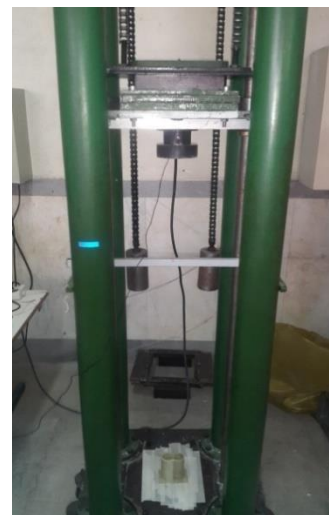
Fig. 2 Impact tests setup using Drop Tower machine
