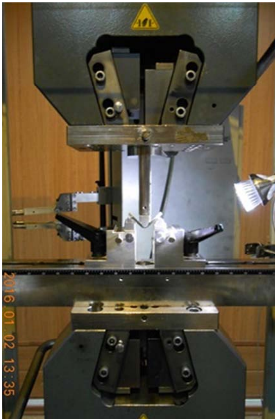
Fig. 8 The three-point bending test set-up.
