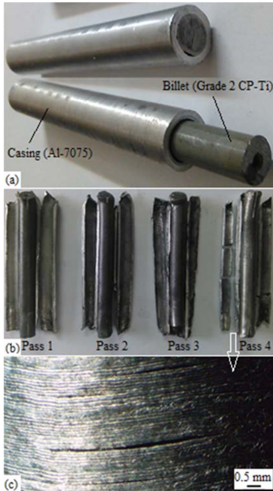
Fig. 5 Bimetallic specimens (a) Before ECAP, (b) After ECAP, and (c) Optical macroscopic image of surface cracks after fourth pass ECAP.
