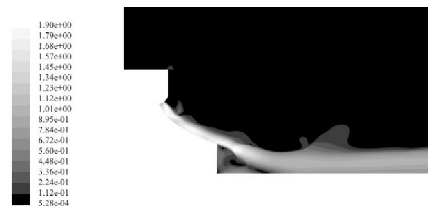
Fig. 11 Contour of Mach number in pressure ratio of 5.2
