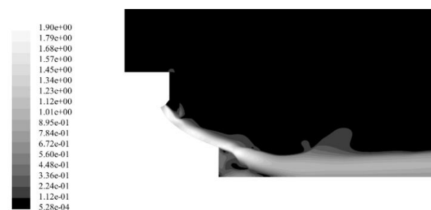
Fig. 11 Contour of Mach number in pressure ratio of 5.2
