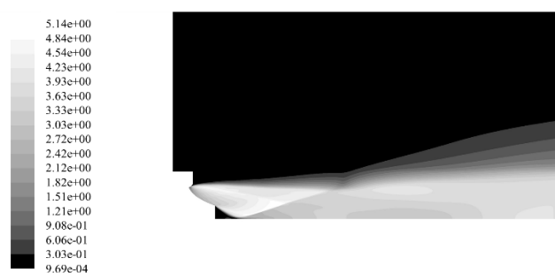
Fig. 13 Contour of Mach number in pressure ratio of 200
