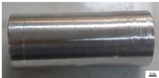
Fig. 3 Casting alloy sample after turning
