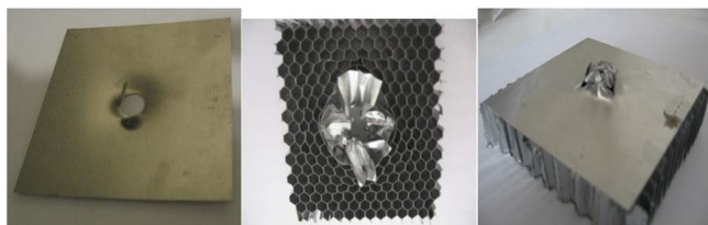
Fig. 7 The backside of specimens, after the quasi-static penetration (From left to right aluminum plate, honeycomb structure and sandwich panel)
