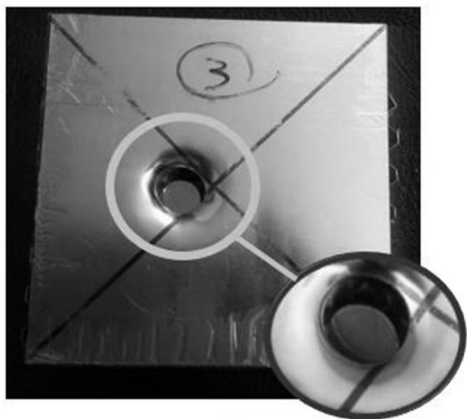
Fig. 17 An example of the projectile stuck in the sandwich structure
