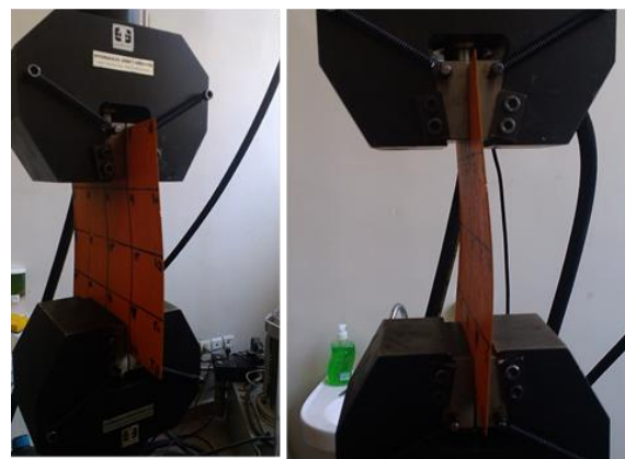
Fig. 1 Glass-fiber laminate under static compression load with constant strain rate 0.005 mm/s
