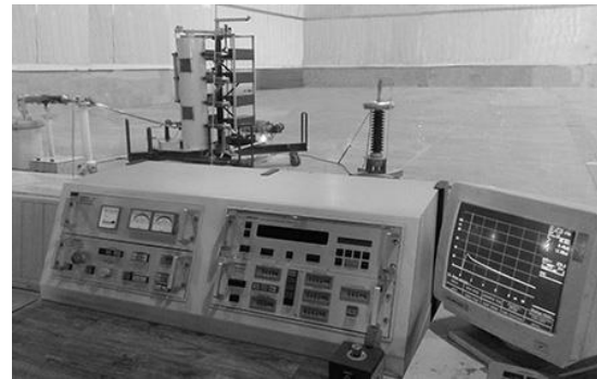
Fig. 5 Electrohydraulic forming apparatus
