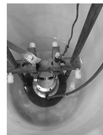
Fig. 6 Electrode system in the water chamber
