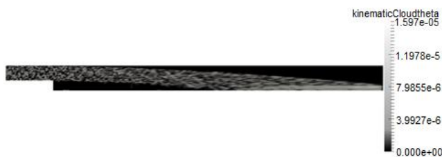
Fig. 11 The volume ratio of particles to the fluid around (gas) after one second in the step problem
