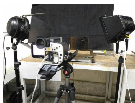
Fig. 4 Experimental set-up used to thermography
