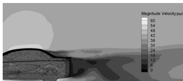
Fig. 18 distribution of velocity on the model with spoiler
