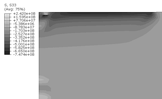
Fig. 6 Radial residual stress field (Pa) for single laser shot peen
