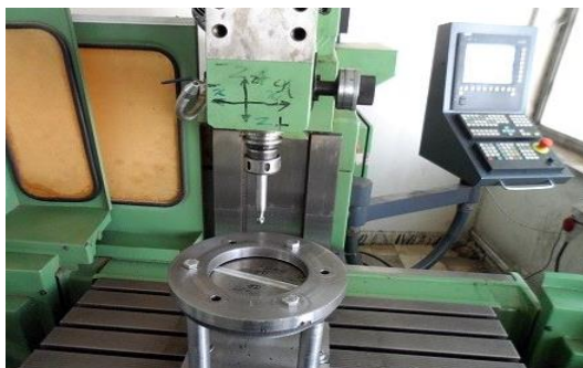
Fig. 2 The milling machine and fixture used for incremental forming process
