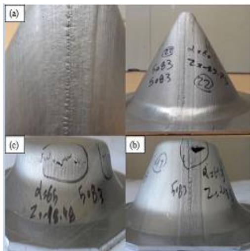
Fig. 7 Incremental forming of friction stir welded 5083 aluminum sheets. (a) 60°, (b) 61.3°, (c) 65°
