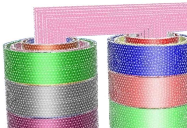
Fig. 14 Close view of transformer meshing
