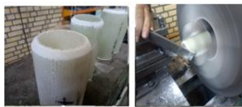
Fig. 7 chamfering the samples with a grinding machine
