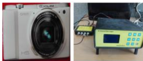
Fig. 10 Data logger and high speed camera
