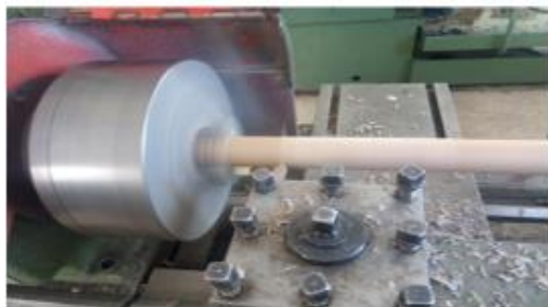
Fig. 4 Mandrel diameter correction with machining
