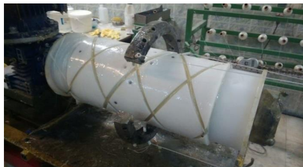
Fig. 5 Fabrication process of stiffeners
