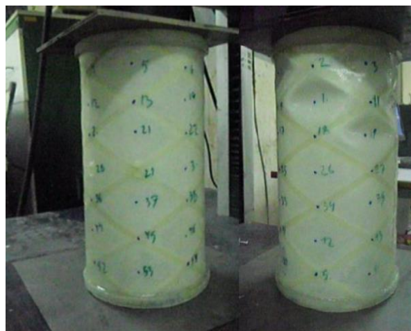
Fig. 12 Specimen before and after buckling
