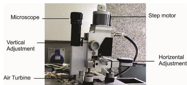
Fig. 2 The device used for high-precision stage punching
