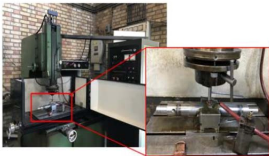
Fig. 7 Spark erosion at mid-span of the specimens
