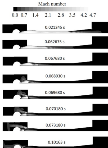
Fig. 13 Contours of Mach number in computational domain during motor terminating phase
