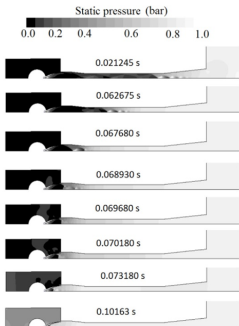
Fig. 15 Contours of static pressure in computational domain during motor terminating phase
