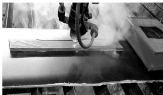
Fig. 11 Precise cutting of PVCU samples using laser cutting machine
