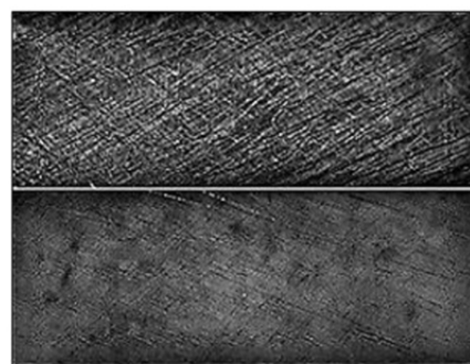
Fig. 28 Failure surfaces of UDCB sample with NCVP209
