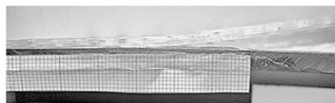
Fig. 27 Crack growth path in the UDCB sample with NCEP25
