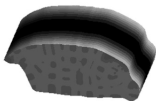
Fig. 6 Uncoupled and coupled 2nd acoustic mode shape contour
