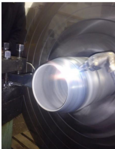
Fig. 6 Experimental configuration of tube spinning.
