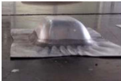
Fig. 5 A deformed part after deep drawing process
