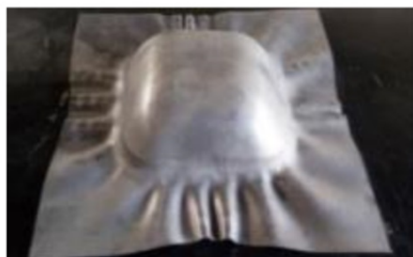
Fig. 9 The wrinkled specimen from experiment No. 1
