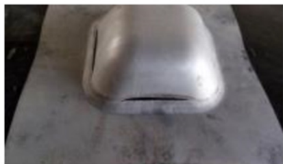
Fig. 10 The ruptured specimen from experiment No. 16
