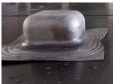
Fig. 6 A deformed part after gas forming process
