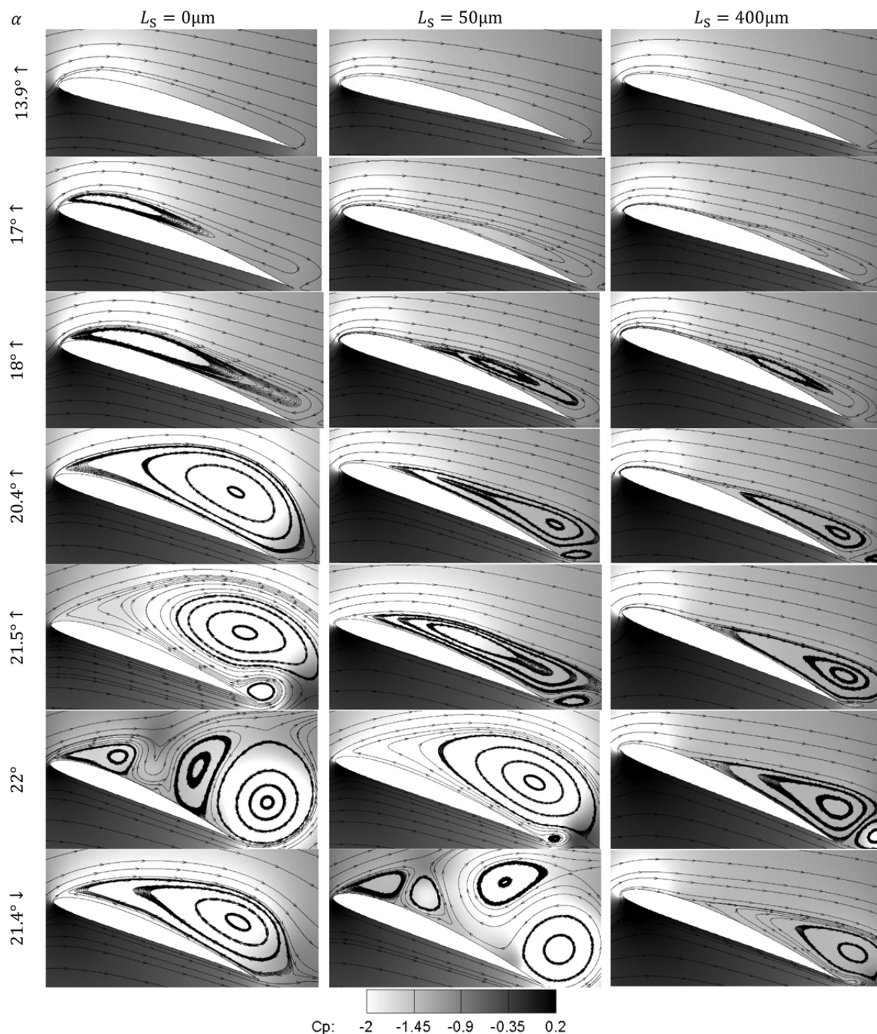
Fig. 12 Governing pressure field structure at oscillating cycle superimposed by streamlines.
