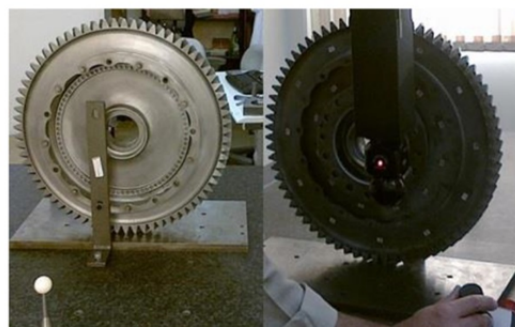
Fig. 4 disc dimension measurements by coordinate measurement machine (CMM)
