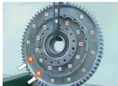
Fig. 1 Investigated disc and points of response measurements
