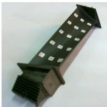
Fig. 2 specified points for modal testing of blade
