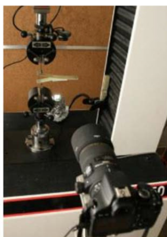
Fig. 2 DCB specimen is being tested
