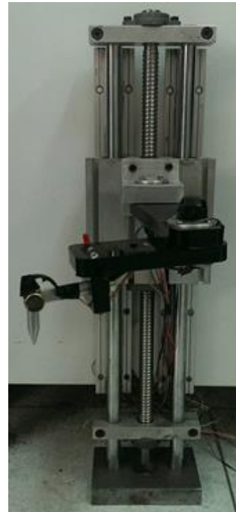
Fig. 4) Constructed prototype of SA_PeD: the base, arms, end-effector and optical alarms.
