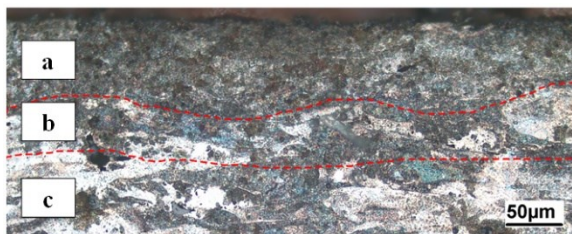
Fig.4 Three key zones formed by the shot-peening process on the part surface: (a) shot-affected zone, (b) transition zone, (c) unaffected zone
