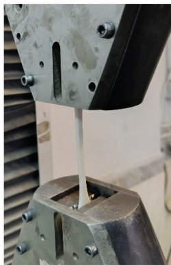
Fig. 6 uniaxial tensile test for extracting mechanical properties
