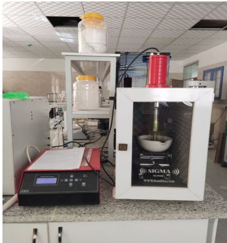
Fig. 1: The ultrasonic setup utilized for dispersion of nanoparticles into the base material.
