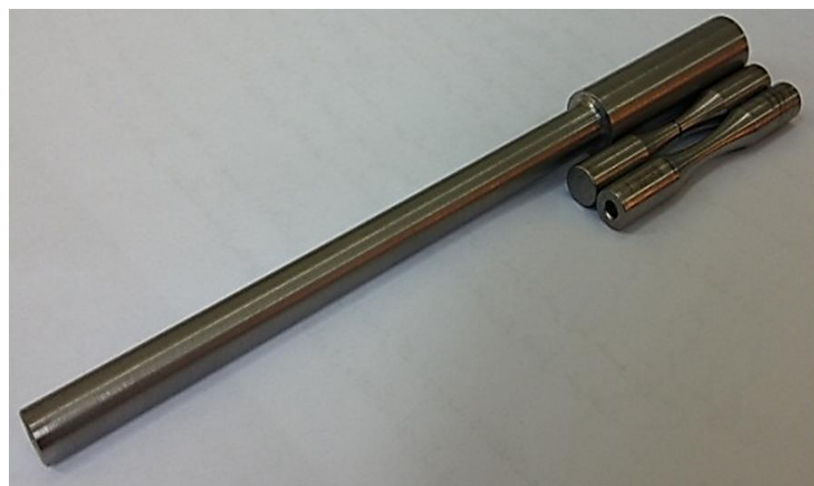
Fig. 4 Specimens used for fatigue tests
