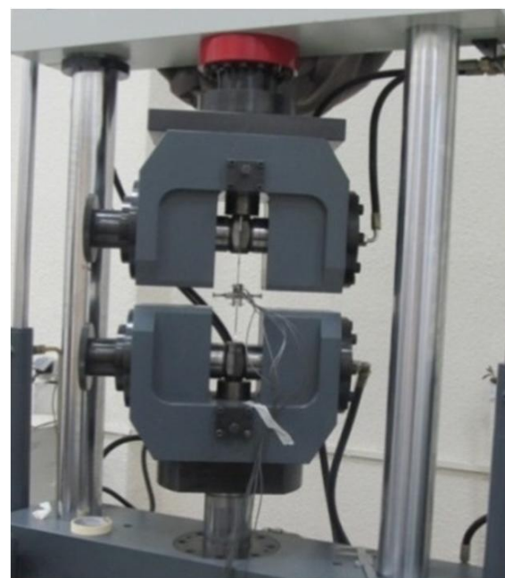
Fig. 5 fretting fatigue test assembly in fatigue machine
