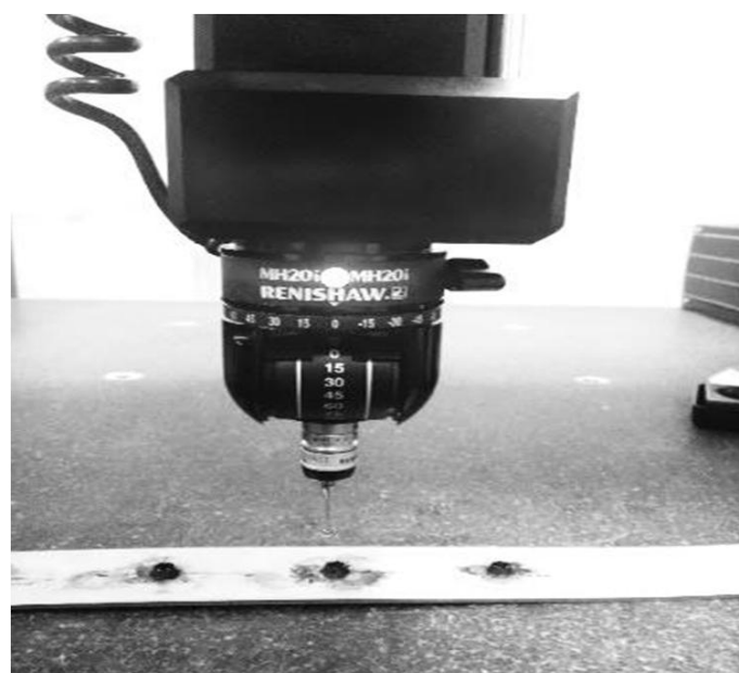
Fig. 6 Measurement of bush length by CMM
